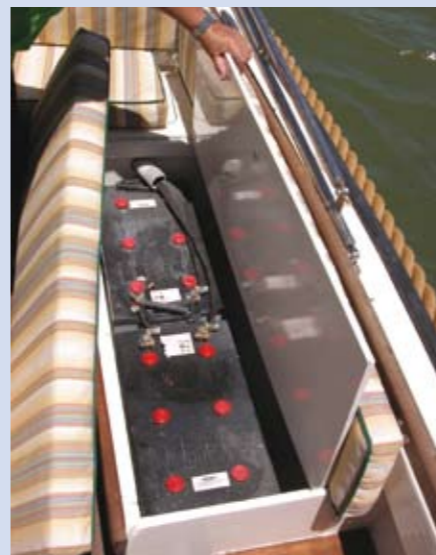
Clockwise from below left: Four 180-amp semi-traction batteries, stored in pairs under the aft side seats, provide enough juice for about six hours of silent cruising; there's an automatic fire extinguisher in the engine compartment, with backup from a portable unit; a stainless steel alcohol-burning stove and fresh water basin are among the mod-cons. Bottom: The diesel engine can be used to drive the electric motor, turning it into a dynamo to charge the batteries.
