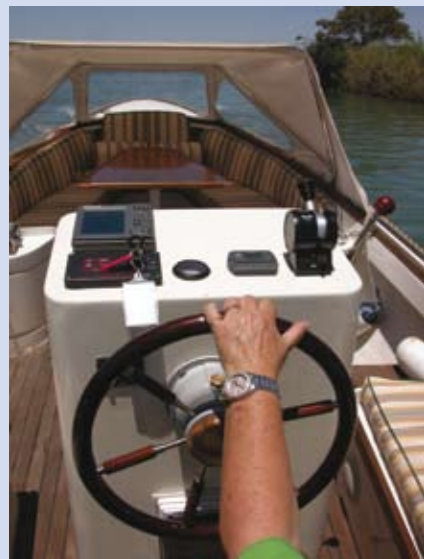
Clockwise from top: Large, well-positioned windows in the spray hood provide plenty of forward vision for those seated at the helm. Seating eight in comfort, the cockpit's height of 68 cm provides sufficient passive safety for small children. The brushless 2,2 kW electric motor delivers a maximum speed of 4,8 knots (9 km/h).
